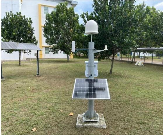
Faculty of Electrical and Electronics Engineering Technology Solar System (weather/rain/irradiation data collector system) takes data and sends it directly to the server using IoT technology, solar is used as a continuous energy source 24/7.
